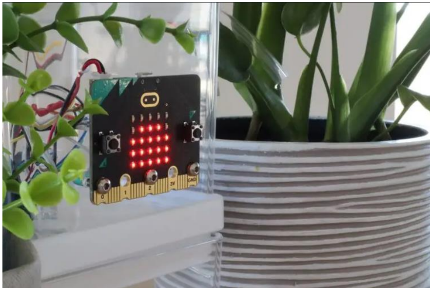
Figure 34: Acrylic case for Micro:bit-based automatic watering system (Image from: https://www.instructables.com/Automatic-Plant-Watering-System-Using-a-Microbit/ )
